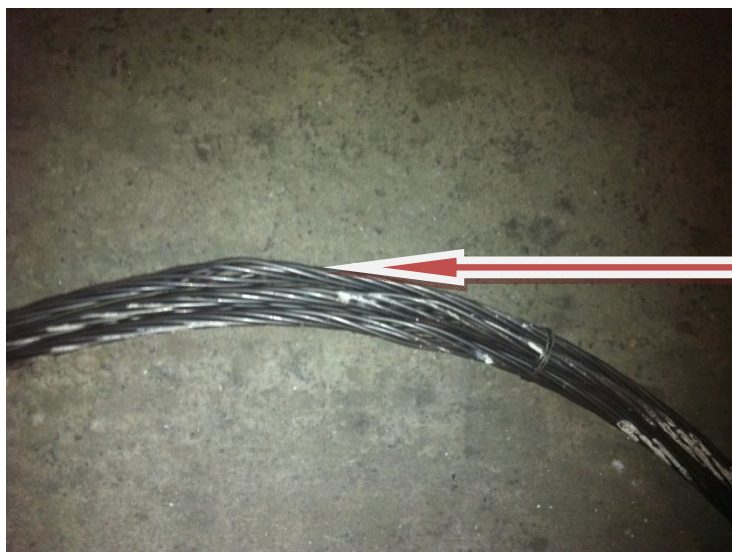
The cable strand is made up of braided metal wire
