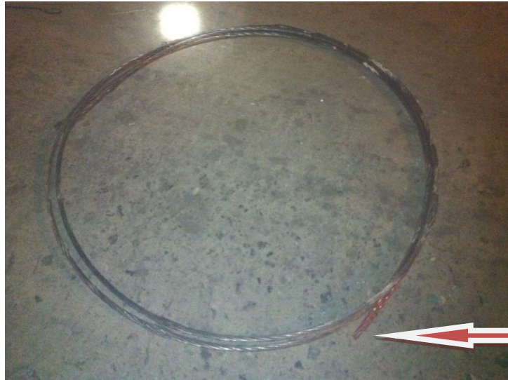
Single strand Cable Bolt 10m in length
